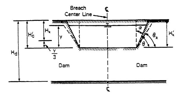
Figure 4: Front View of Dam with Breach
