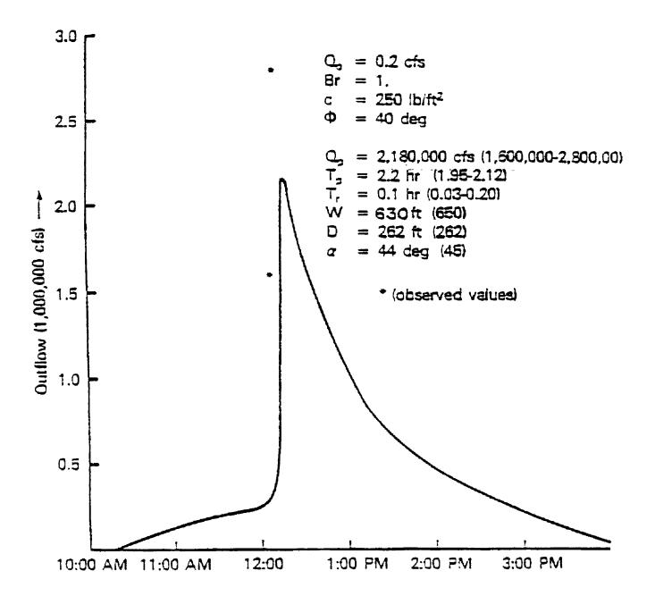
Figure 6: Teton Dam: Predicted and Observed Breach Outflow Hydrograph and Breach
