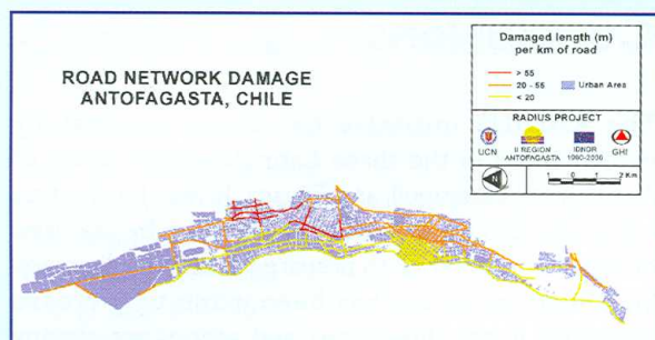
Figure 3. Road damage estimated for Antofagasta, Chile.
