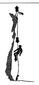
Unassisted belay, done using an ascender 1.5kN (153kgf)
