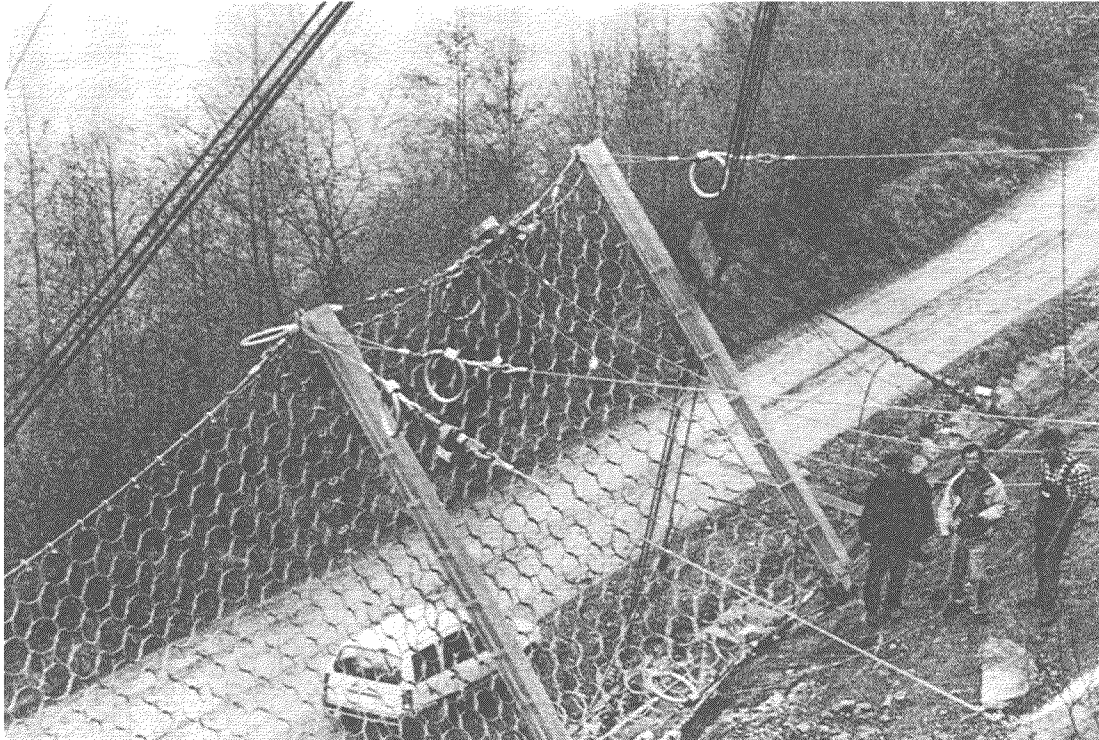
Fig.4.3 Rockfall Barrier with Brake Rings and Strain Gauges.
