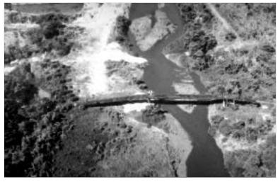
d Pipelines tha cross rivers or ravines should be designed to accomodate flood levels.
