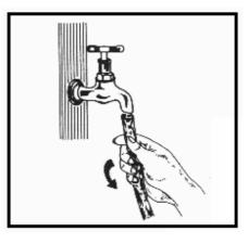
b) Open the faucet and let the water flow for one to two minutes, before collecting the sample. This procedure cleanses the opening and flushes out water which has collected in the pipe.
