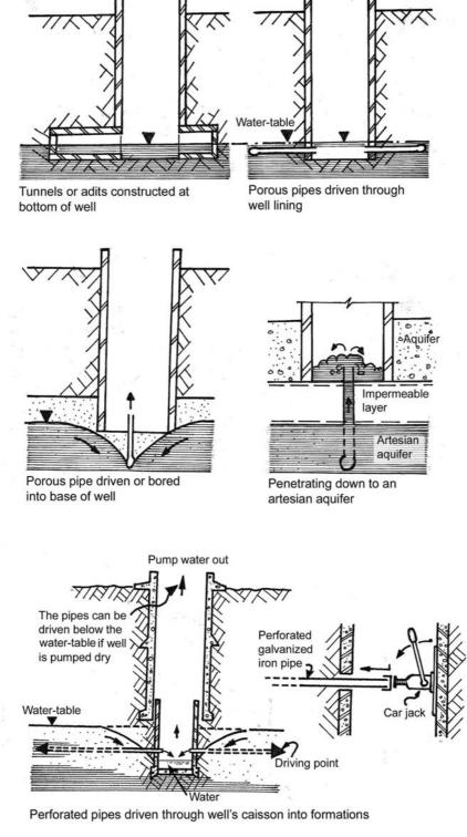
Figure 7.10 Methods of improving the output of wells<sup>1</sup>
