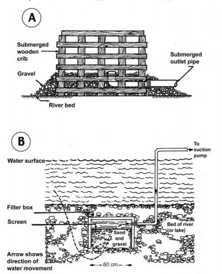
Figure 7.14 Water intake systems for lakes or rivers: (A) Wooden crib at intake; (B) Lake or river-bed filter<sup>1</sup>
