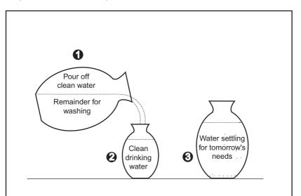
Figure 7.16 Simple household storage system for removal of sediment<sup>1</sup>
