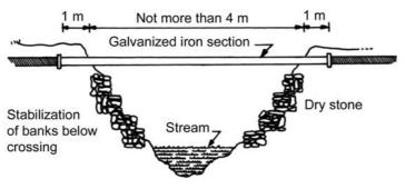
Figure 7.1 Reinforcement of water pipes crossing streams or gullies<sup>1</sup>
