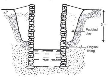
Figure 7.8 Improving an existing well with puddled clay<sup>1</sup>
