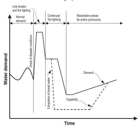
Figure 7.3 Water demand under normal and emergency conditions
