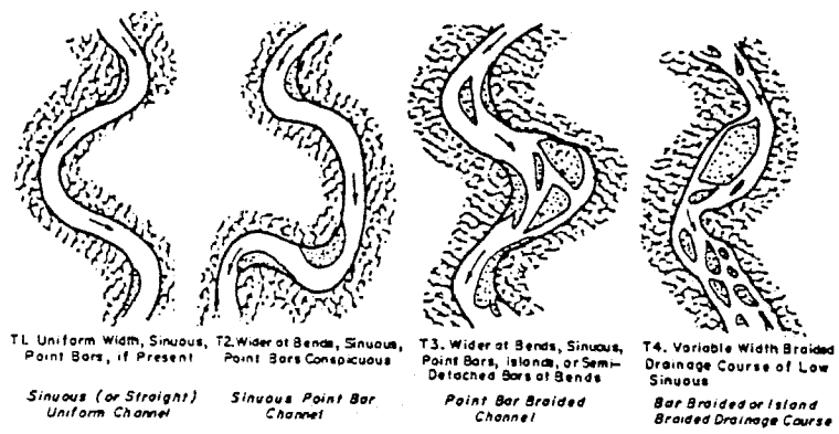
(a) Variability of Unvegetated Channel Width: Channel Pattern at Normal Discharge
