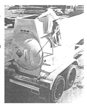
Rubberlined chemical tanker, undergoing inspection at manufacturer's, is painted white to promote heat reflection and will soon be hauling corrosives
