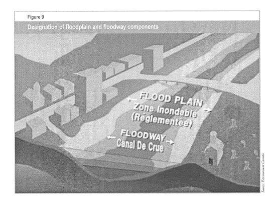
There may be a necessity to define several zones within the flood-prone area, dependent on the velocity of the river and other physical factors. As an example, the flood-prone area may be broken down into floodway and flood plain components. Figure 9 shows a schematic of the designated floodway and flood plain for a hypothetical community.
