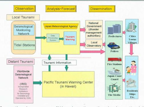
In case of an earthquake occurrence, JMA analyzes the earthquake observational data and quickly issues tsunami warning, if necessary. The warning is automatically transmitted to disaster management authorities and broadcasting media. The earthquake and tsunami information including tsunami warning is used as a trigger of evacuation and urgent operation for rescue and mitigation of disasters.
