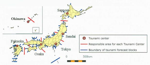
When a large earthquake occurs, the database is searched using the location and magnitude of the earthquake as indices, and the stored heights and arrival times of tsunami along the coasts are read out, for the issue of tsunami warnings for individual 66 tsunami forecast blocks in the coastal area.
