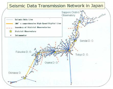
Transmission lines are connected between neighboring centers to share the earthquake data. This network allows for continued monitoring and analyzing of earthquakes, even if part of the network would be damaged by a large earthquake.
