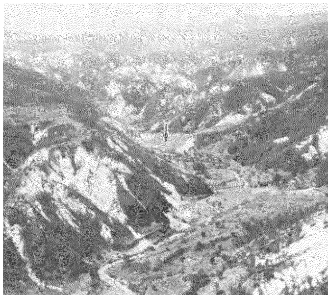
FIGURE 35.—Aerial view looking northeastward along Río Pixcayá, due north of Chimaltenango, showing numerous landslides in pyroclastic deposits. The river was partially dammed by a major landslide, shown by arrow in the middle distance. (Also see fig. 37.)
