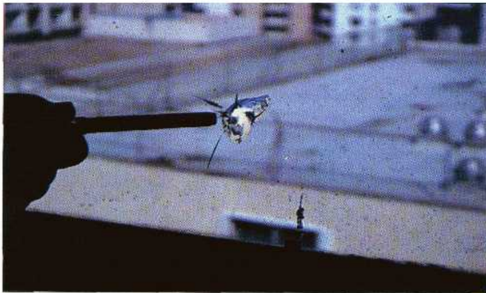
FIGURE 5-25 Although some annealed panes broke into shards, others just broke at the impact point.
