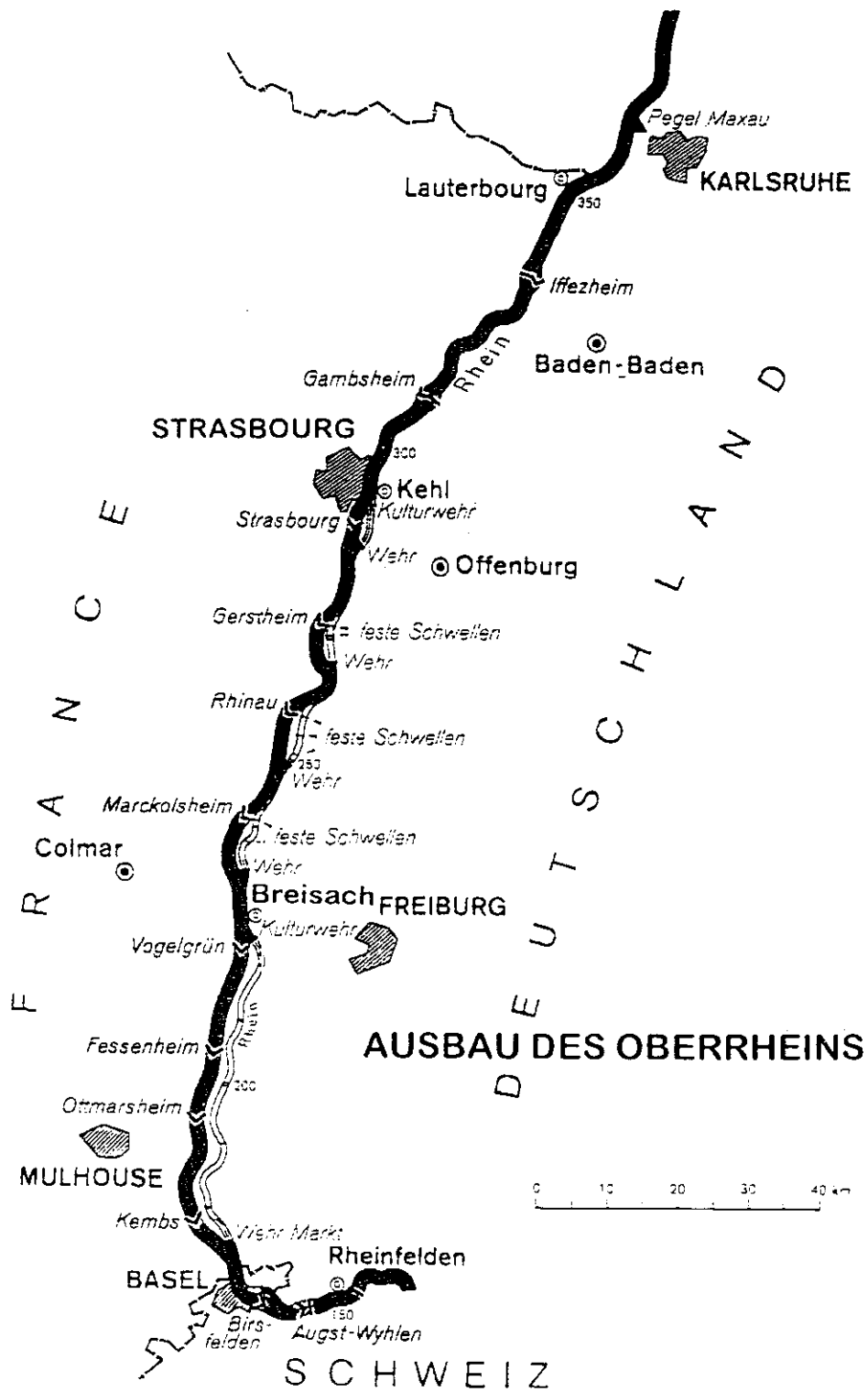
Illustration 1: Ground plan of the barrages along the Upper Rhine
