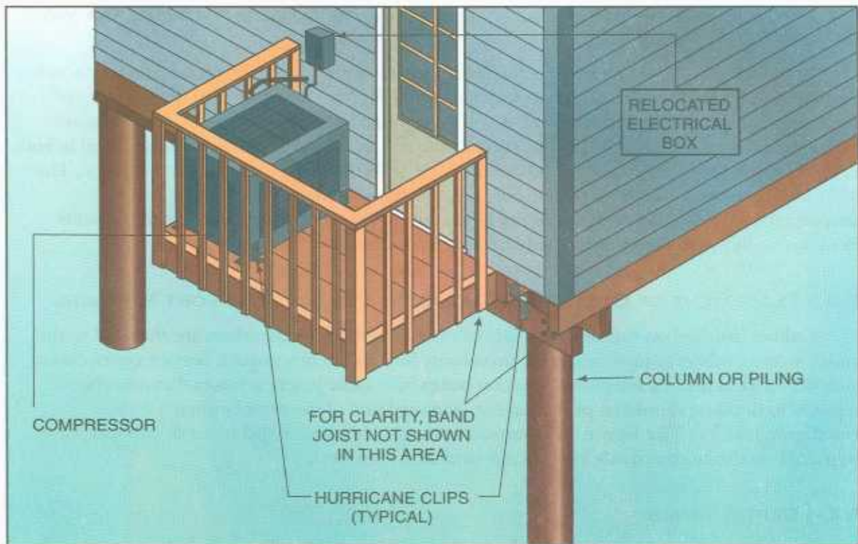
Figure 3-5 Cantilevered mechanical platform.
