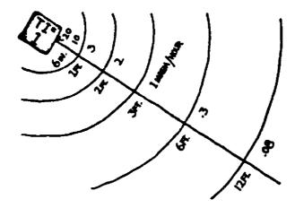
Radiation levels vs. distance from the surface of the package with TI of 1.
