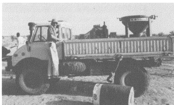
Pesticide ground spreader mounted on a Unimog truck in northern Mauritania
