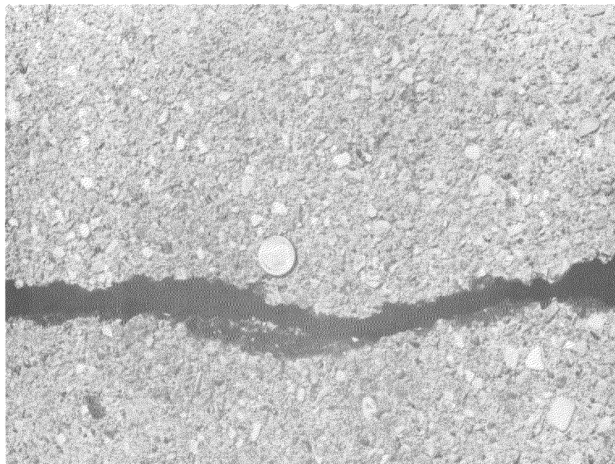
Fig. 9.4 Close up of the extension fracture shown in Fig. 9.3. Scale given by the coin (quarter) in the center of the picture.
