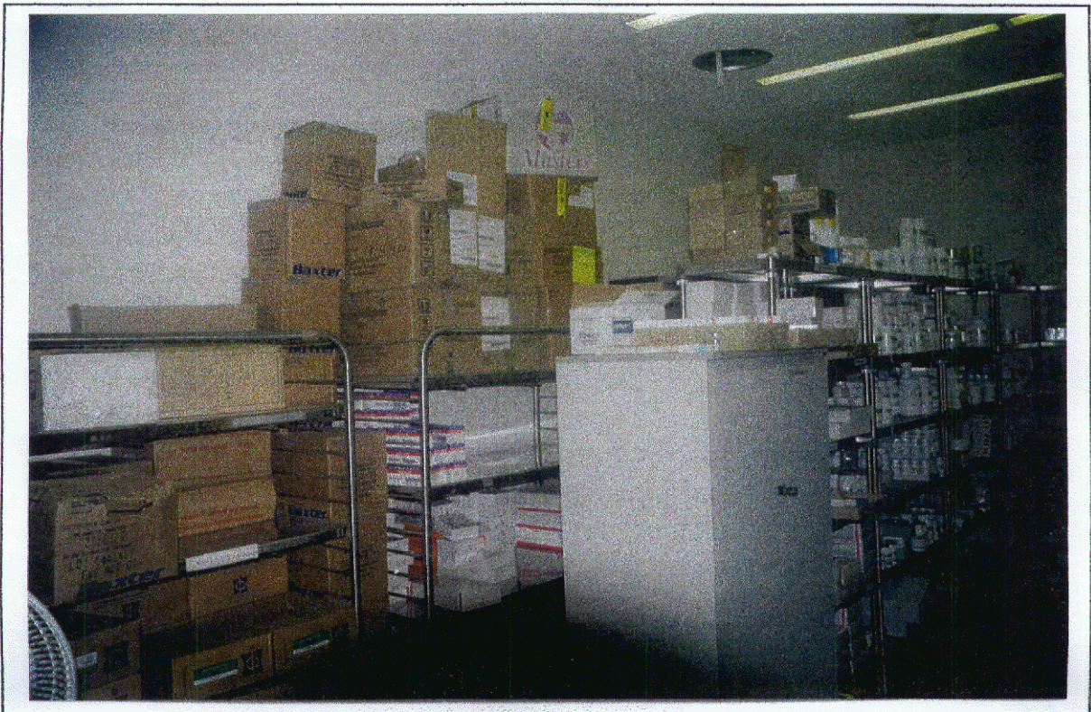
Photo 14 - The storage room of the Laboratory Medical supplies are vulnerable to falling off the shelves in earthquakes
