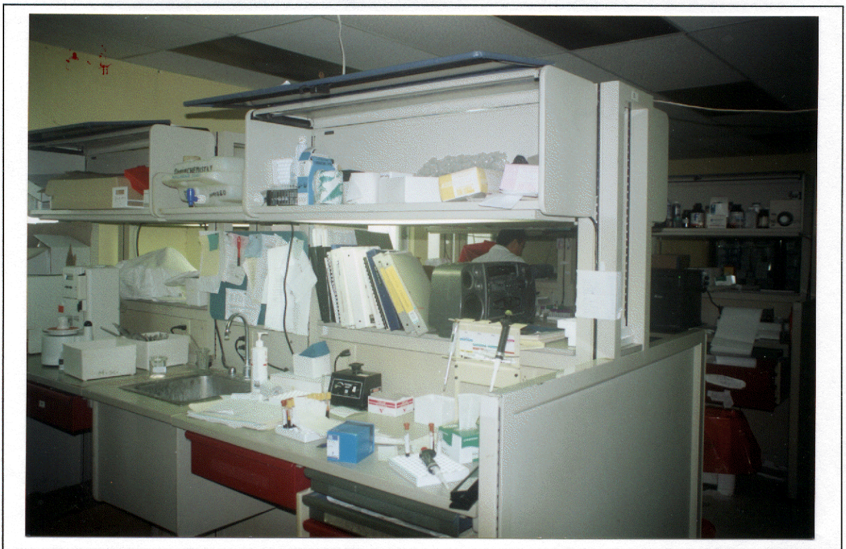
Photo 31 - Chemistry and Haematology High-level cupboards left open Contents are vulnerable in the event of an earthquake.
