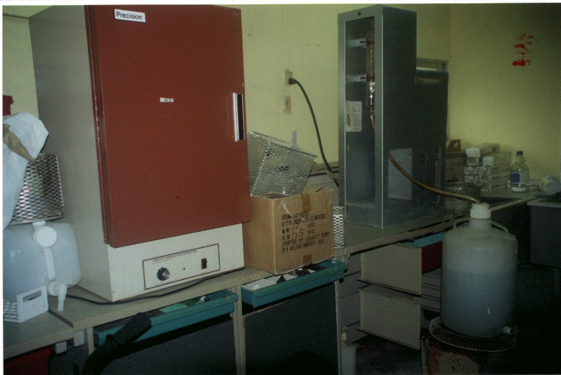
Photo 34 - Wash Room High-level equipment vulnerable to toppling in the event of an earthquake.
