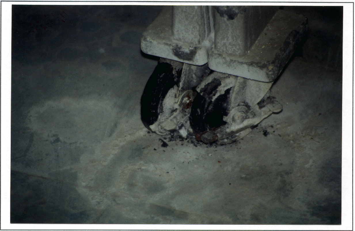
Photo 35 - Equipment on wheels The bakes are unlikely to be operational in the observed condition.
