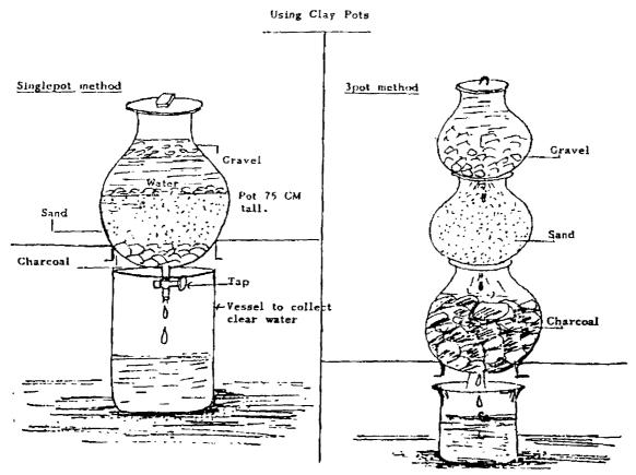
The water is made to pass through sand, gravel or charcoal Bacteria and other pollutants are removed.
