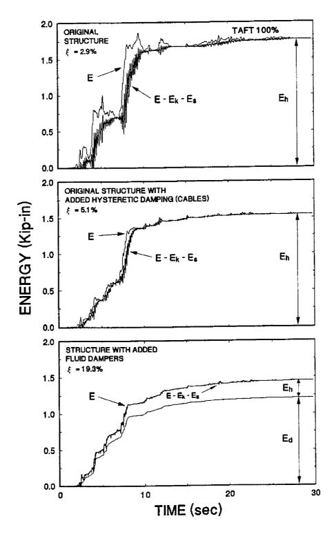
FIGURE 5-3 Energy Time Histories in One-story Stiffened Structure Subjected to Taft 100% Motion (1 Kip = 4.46 KN, 1 in. = 25.4 mm)
