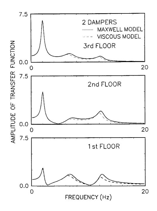
FIGURE 4-4 Comparisons of Amplitudes of Transfer
