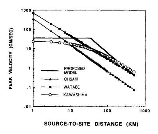
Fig.7-2 Comparison of Proposed Model with Currently Existing Models from Japan for Magnitude 7.0 Earthquake
