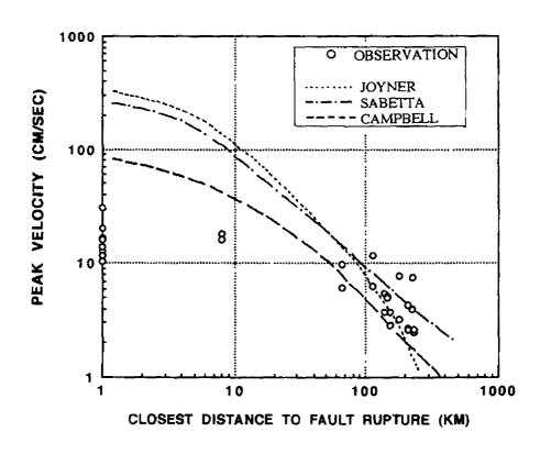
Fig.8-13 Comparison of Observed Peak Velocity at Rock Sites for the 1985 Michoacan Earthquake with Empirical Estimates for a Magnitude 8.1 Event by Joyner and Boore, Campbell and Sabetta
