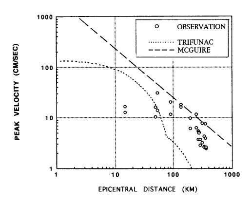
Fig.8-12 Comparison of Observed Peak Velocity at Rock Sites for the 1985 Michoacan Earthquake with Empirical Estimates for a Magnitude 8.1 Event by Trifunac and McGuire
