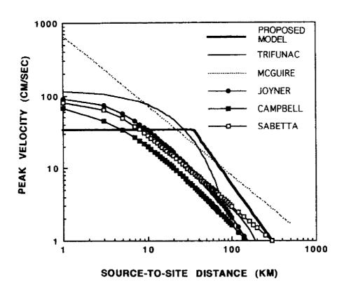
Fig.7-1 Comparison of Proposed Model with Currently Existing Models from the US. and Italy for Magnitude 7.0 Earthquake
