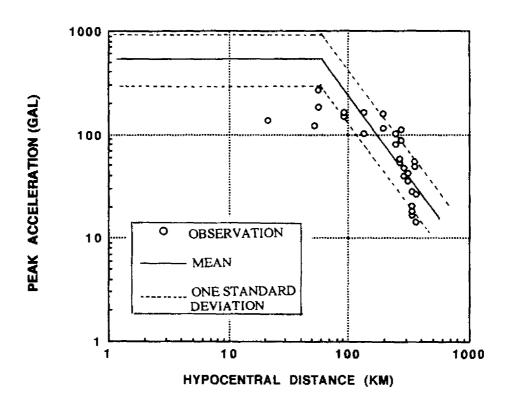
Fig.8-4 Comparison of Peak Acceleration at Rock Sites for the 1985
