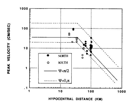
Fig.8-16 Peak Velocity at Rock Sites for the Loma Prieta Event with Scatter Bands Based upon Rupture Directivity in Fig.8-15
