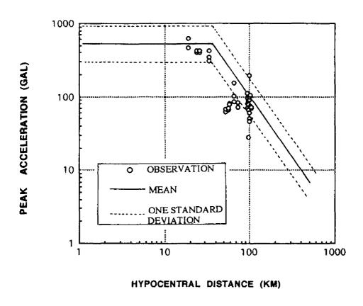
Fig.8-1 Comparison of Peak Acceleration at Rock Sites for the 1989 Loma Prieta Earthquake with Value Predicted by the Proposed Semi-Empirical Model for M=7.0
