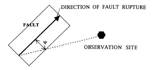
Fig.8-15 Sketch showing Azimuth Angle for an Arbitrary Observation Site with Respect to the Direction of Fault Rupture
