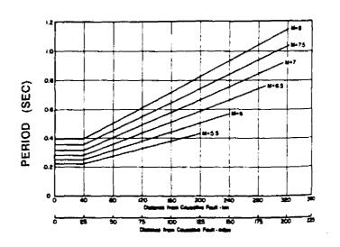
Fig.6-4 Predominant Periods for Acceleration on Rock (after Seed et al.[25])
