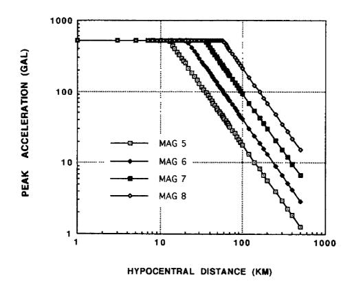
Fig.6-1 Attenuation Relationship for Peak Acceleration on Bed Rock from Proposed Semi-Empirical Model
