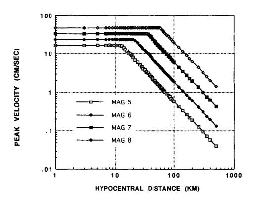
Fig.6-2 Attenuation Relationship for Peak Velocity on Bed Rock from Proposed Semi-Empirical Model
