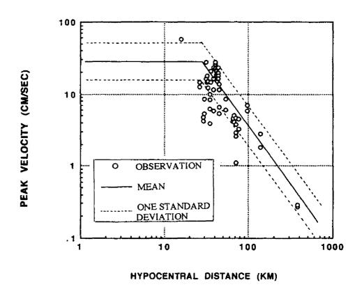
Fig.8-8 Comparison of Peak Velocity at Rock Sites for the 1971 San Fernando Earthquake with Value Predicted by the Proposed Semi-Empirical Model for M=6.6
