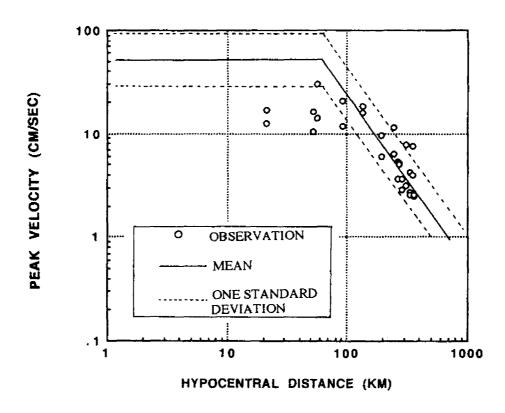
Fig.8-5 Comparison of Peak Velocity at Rock Sites for the 1985 Michoacan Earthquake with Value Predicted by the Proposed Semi-Empirical Model for M=8.1
