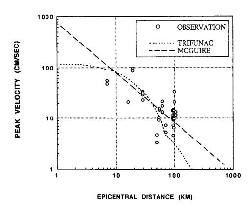
Fig.8-10 Comparison of Observed Peak Velocity at Rock Sites for the 1989 Loma Prieta Earthquake with Empirical Estimates for a Magnitude 7.0 Event by Trifunac and McGuire
