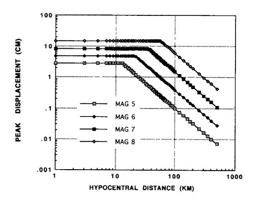
Fig.6-3 Attenuation Relationship for Peak Displacement on Bed Rock from Proposed Semi-Empirical Model
