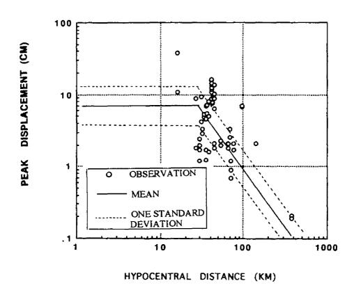
Fig.8-9 Comparison of Peak Displacement at Rock Sites for the 1971 San Fernando Earthquake with Value Predicted by the Proposed Semi-Empirical Model for M=6.6
