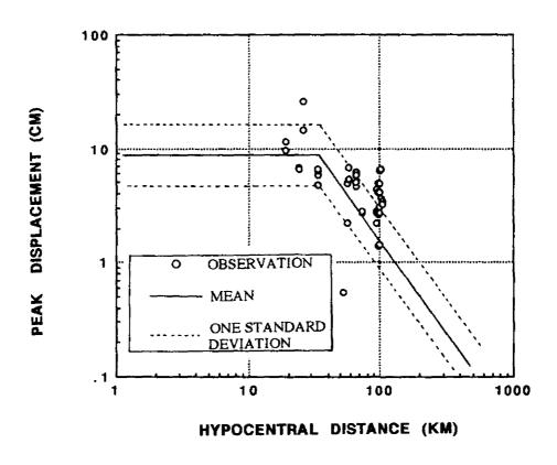
Fig.8-3 Comparison of Peak Displacement at Rock Sites for the 1989 Loma Prieta Earthquake with Value Predicted by the Proposed Semi-Empirical Model for M=7.0
