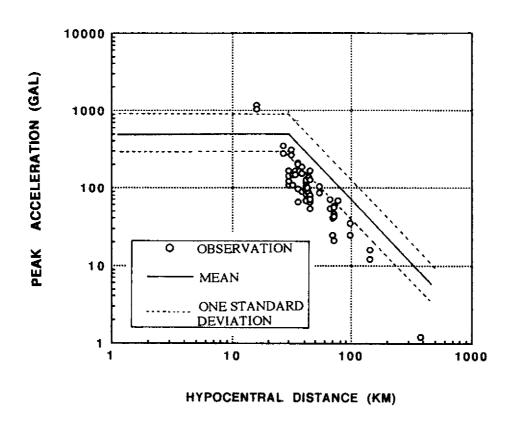
Fig. 8-7 Comparison of Peak Acceleration at Rock Sites for the 1971 San Fernando Earthquake with Value Predicted by the Proposed Semi-Empirical Model for M=6.6
