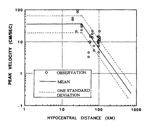
Fig.8-2 Comparison of Peak Velocity at Rock Sites for the 1989 Loma Prieta Earthquake with Value Predicted by the Proposed Semi-Empirical Model for M=7.0
