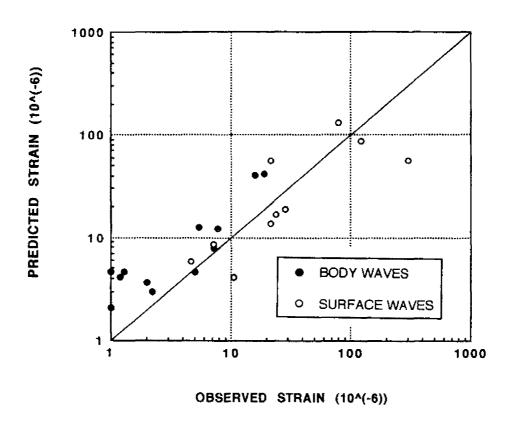
Fig.9-6 Comparison Between Observed Soil Strain at the Kubota Corp. Shimonaga Site and Predicted Values from Eqs.(9.3) or (9.4)
