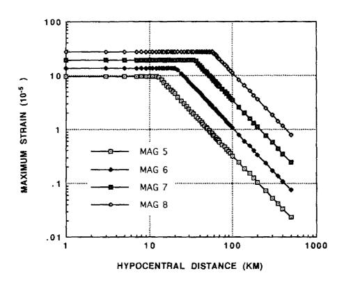
Fig.9-2 Attenuation for Estimated Maximum Soil Strain at Rock Site Subject to Surface Waves
