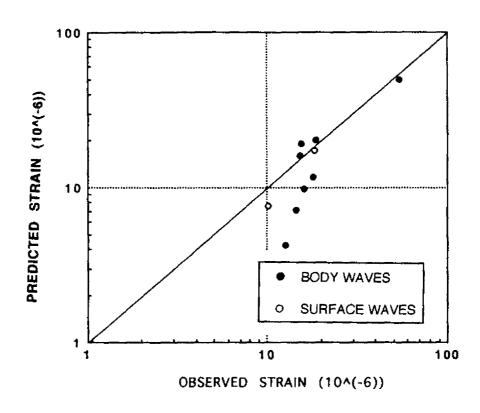
Fig.9-7 Comparison Between Observed Soil Strain at the Univ. of Tokyo Chiba Site and Predicted Values from Eqs.(9.3) or (9.4)
