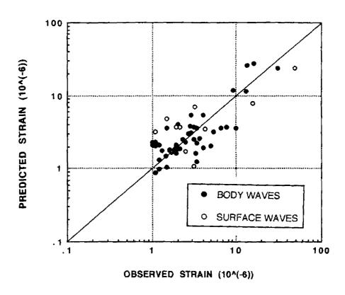
Fig.9-5 Comparison Between Observed Soil Strain at the Kubota Corp. Kansen Site and Predicted Values from Eqs.(9.3) or (9.4)
