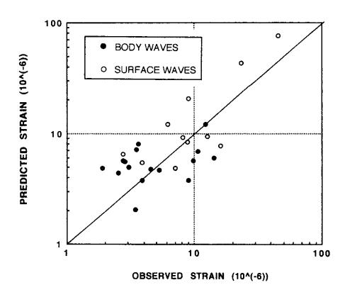
Fig.9-8 Comparison Between Observed Soil Strain at the Chubu Electric Power Corp.Chubu Site and Predicted Values from Eqs.(9.3) or (9.4)
