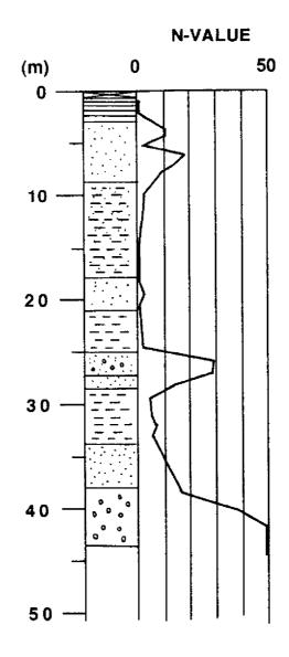
Fig.9-4 Soil Profile for the Shimonaga Site (Kubota Corp. Soil Strain Installation)
