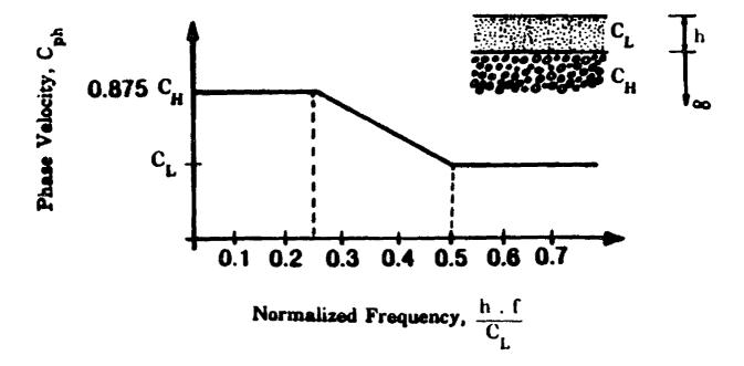
Fig.9-1 Approximate Dispersion Curve for Fundamental R-wave for Uniform Soil Layer over a Half Space( after O'Rourke et al.[38])
