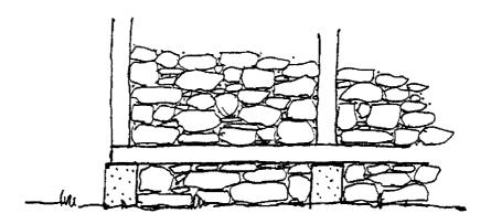
The mortar of the older stone nog buildings was often made of mud, burnt marl, and fibers such as horse hair. More recently, lime and mud or cement and sand mortars have been used. The sand and cement mortars have weathered well, but the lime and mud show much deterioration.
