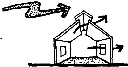
Vent openings can be on outside walls, or on roof.
