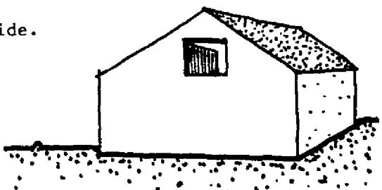
Use a vent on the top of the roof
