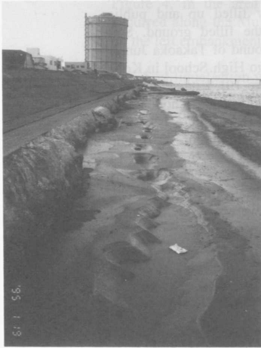
Photo 28 Sand boils along Torishima Dike of Yodo River (Courtesy of Mr. R. Isoyama)
