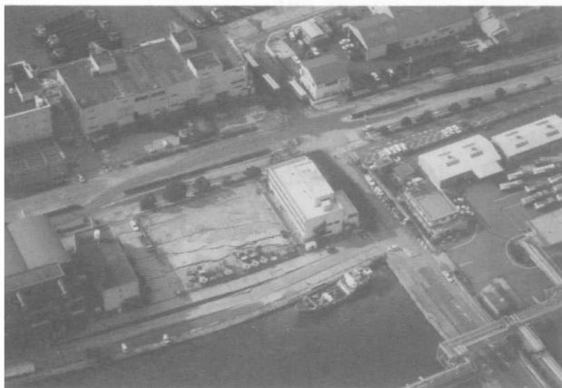
Photo 53 Curved quaywall along due to lateral ground movement toward the sea at road for Maya Wharf
