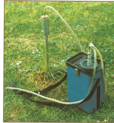
A radon emanometer, an instrument which counts alpha particles.
