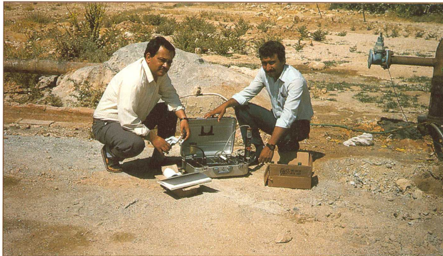
Sampling groundwater during a radon survey in Jordan
