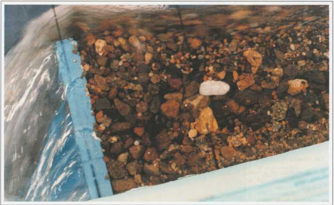
FIGURE 4.9 Hydraulic model study to demonstrate the effectiveness of a check dam in retaining large boulders. Location: Ibaragi, Japan Photo: M. Watanabe
