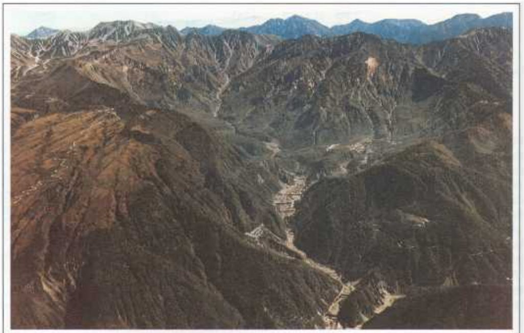
Figure 4.7 Check dams to stabilize the mobile material along a river valley.
