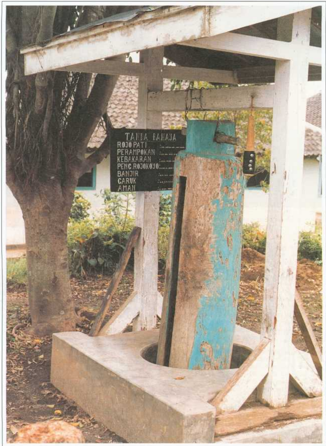
FIGURE 8.8 Example of a tong-tong, a device used for lahar warning in Indonesia. Photo: M. Watanabe.
