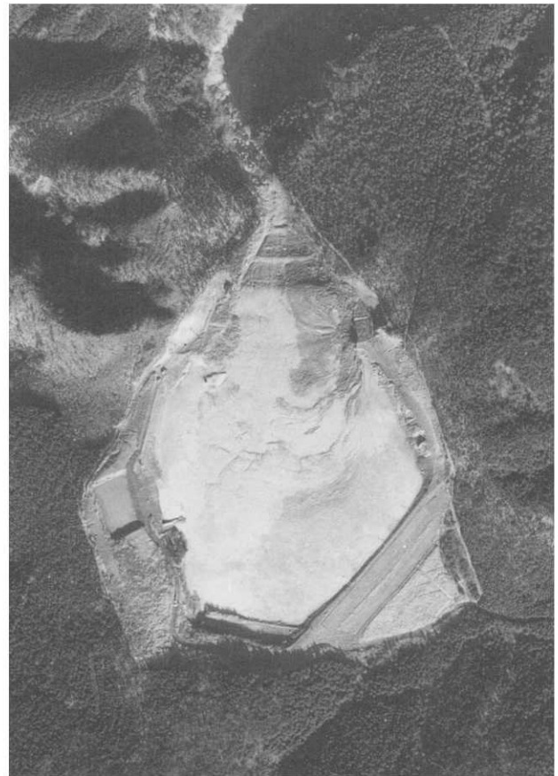
FIGURE 8.24 Hozuki Valley: Collapse of sludge dam No. 1. Photo: S. Hatano.
