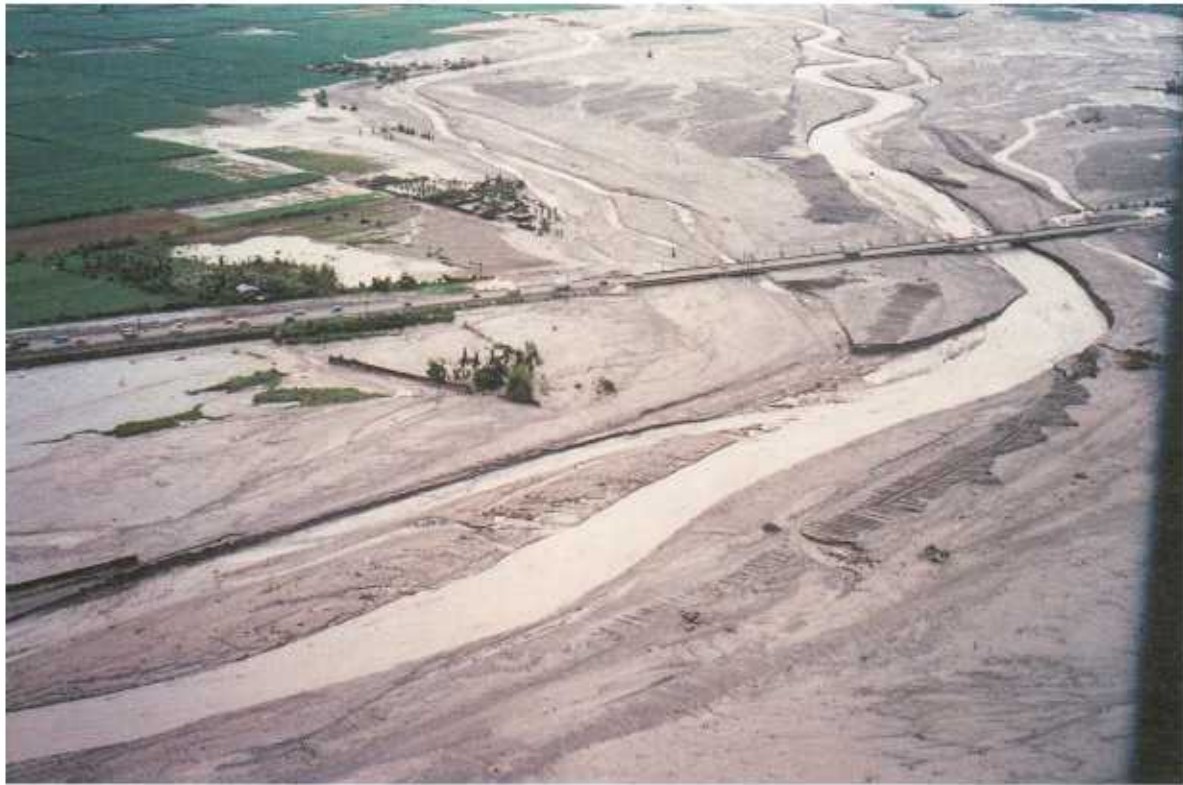
FIGURE 8.47 Mt. Pinatubo. Lahar in the lower reaches of the fan causing widespread damage to the infrastructure. Photo: M. Watanabe.
