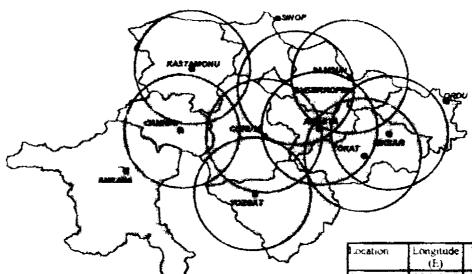
The figure shows theoretical detection capability for small carthquakes, a circle with a radius of 80 km is drawn, with its center located at each local station. An earthquake with a magnitude  $M \ge 3.0$  occuring within the circle is detectable at the station, according to previous research.
