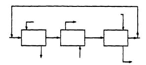
Lines are usually used to represent streams and boxes may be used to represent equipment.
