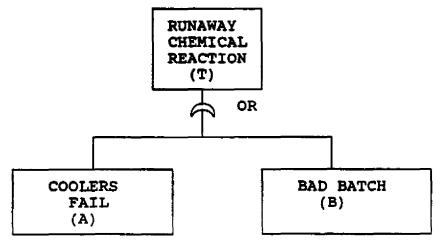
3. Obtain the second branch of the fault tree, applying the logic gates.
