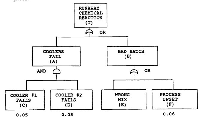
4. Obtain the third branch of the fault tree, applying the logic gates.
