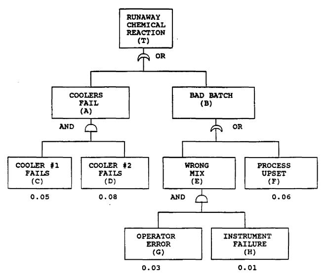
5. Calculate the probability that the runaway reaction will occur.
