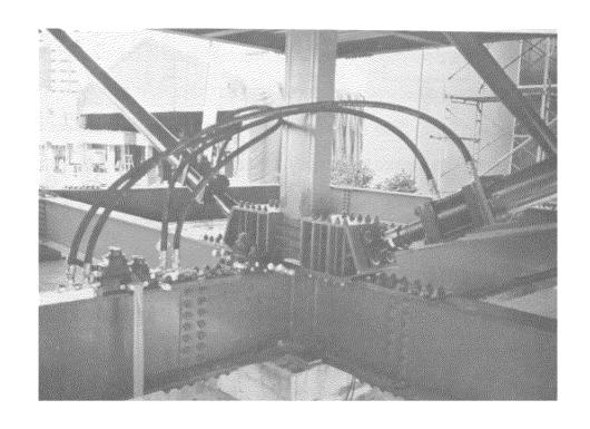
Fig 2.9 A Set of Actuators with a Servovalve
