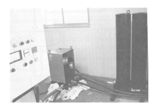
Fig. 2.11 Manifold and Accululators
