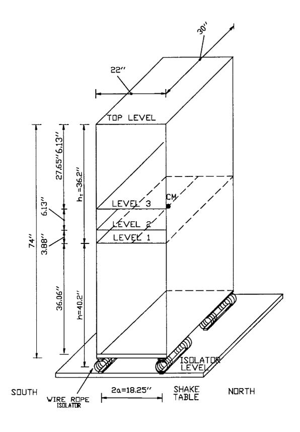
Figure 3-1 Tested Equipment Cabinet (1 in.= 25.4 mm).
