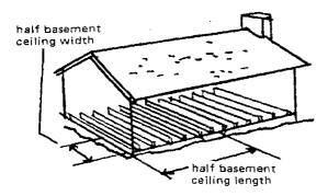
Important: This plan (like Plan A) should not be used if 12 inches or more of your basement wall is above ground level, unless you add the "optional walls" inside your basement that are shown in the Plan A sketch.
