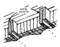
This is similar to Plan A, except that new extra joists are fitted into part of the basement ceiling to support the added weight of the shielding (instead of using a beam and a screwiack column).
