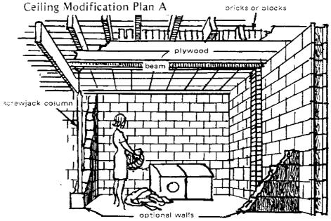
if nearly all your basement is below ground level, you can use this plan to build a fallout shelter area in one corner of it, without changing the appearance of it or interfering with its normal peacetime use.
