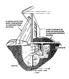
You can add to the protection by making a lean-to over the entrance trench, using boards or house doors, covering them with soil, and covering this with a polyethylene sheet to keep out rainwater.
