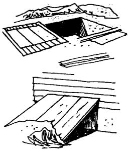
On the doors, pile 12 to 18 inches of earth or sand. Stack or pile other shielding material at the sides of the doors, and also on the other side of the house wall (to protect you against radiation coming from that direction).
