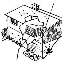
Increase thickness of shelter wall facing exposed basement wall by four inches
