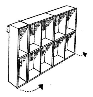
A tilt-up storage unit in the best corner of your basement is another method of setting up a "preplanned" family fallout shelter.
