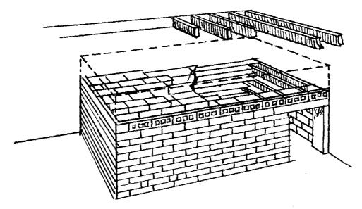
This shelter will provide excellent protection, and can be constructed easily in most parts of the country.
