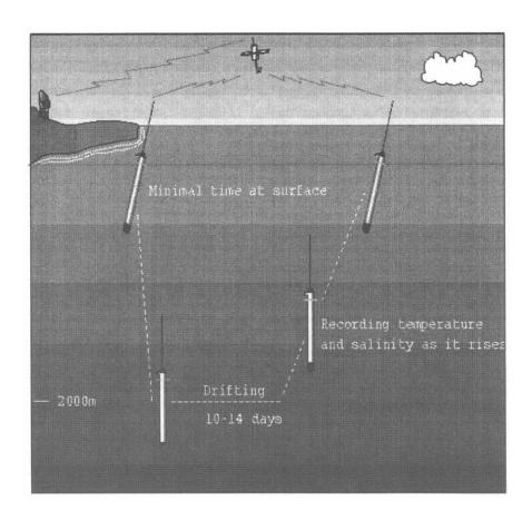
Schematic diagram of the deployment of the Argo float
