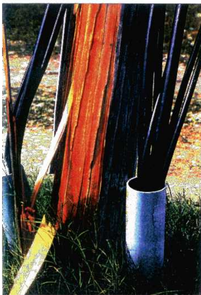
46 Failure of southern-yellow-pine pole due to overstress
