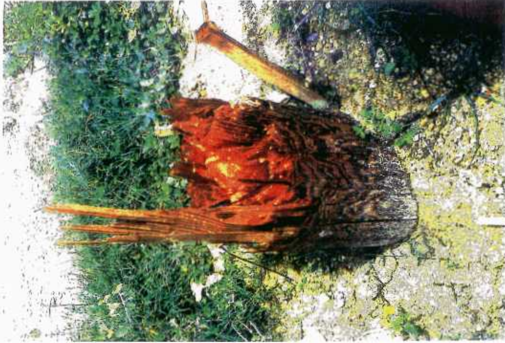
47 Failure of new southern-yellow-pine pole due to overstress
