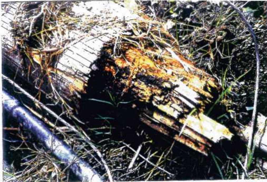
42 Failure of southern-yellow-pine pole due to rotting at the soil line
