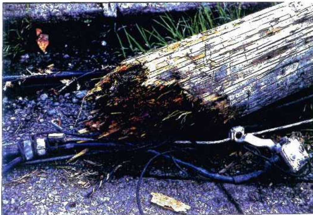
43 Failure of southern-yellow-pine pole (Mental Hospital Road) due to rotting at the soil line
