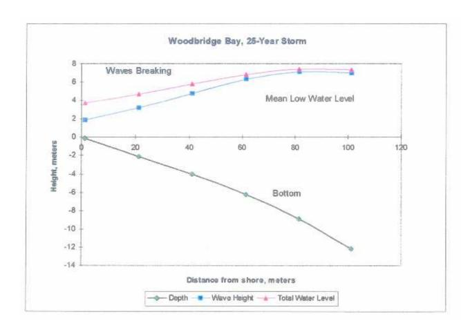
Morne Daniel is a problem area. The cliffs force the coastal road right to the edge of the water, and the underwater configuration brings deep water close to shore. For moderate storms, the rocks north and south of the sample transect help form a buffer. This profile for the 25-year storm shows how that buffer is beginning to be flooded. Waves break 90 meters offshore, and attenuate, but the curves almost level out towards the end.
