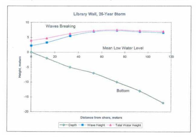
The shore at the library wall, and for some distance north and south of the library, has a uniform slope with few indentations either in this profile or in the plan view. (See site map on page 15.) The storm waves begin to break at about 75 meters from shore, where the total wave height reaches its maximum. The waves steadily lose height and energy as they approach the shore, but there is enough of them left at the shoreline to do damage.
