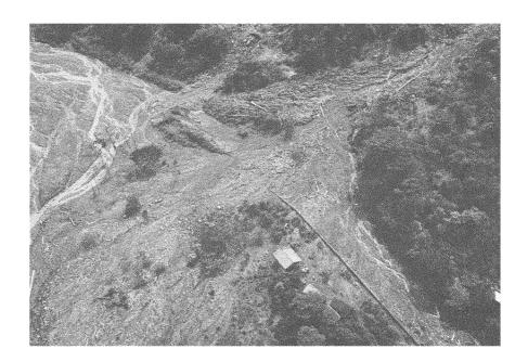
FIGURE 1.8 Aerial view of destruction of the Trans-Ecuadorian oil pipeline and adjacent highway by a debris flow issuing from a minor tributary of the Coca River. Location is near mouth of the Reventador River.
