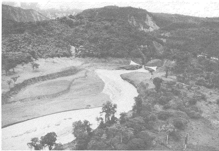
FIGURE 5.20 Downstream view of the Salado River showing location of bedrock constriction (arrows) that caused short-lived damming of the river. Note trimline in jungle cover along lower left valley wall upstream of the river constriction. This trimline indicates the maximum height (about 10 m above current river level) to which the debris flood rose.
