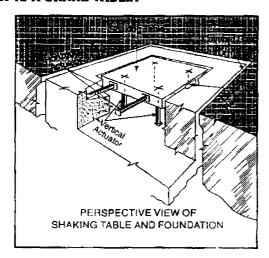
To study the effects of earthquakes on structures, researchers at the National Center for Earthquake Engineering Research (NCEER) mechanically recreate these natural disasters in their laboratory at the State University of New York at Buffalo (UB) using an earthquake simulator or shake table.
