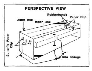
This shaker board consists of a box (with flaps cut off) and an inner box insert that will be the floor of the shaker board. The movement of the shaker board is done by pulling on the kite string from each end and underneath the box. The rubberbands also help simulate movement and shaking. The illustration shows the shake table.
