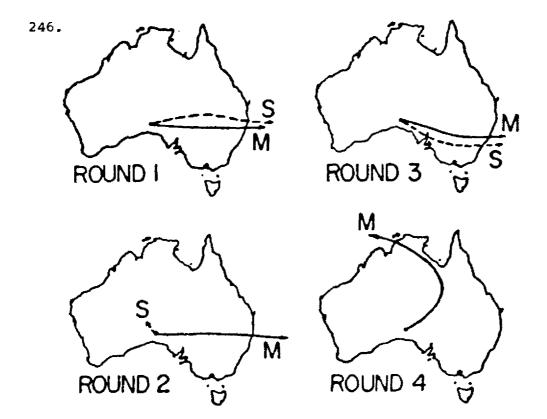
The cloud trajectories are shown for the four explosions. The path of the main cloud (M) is represented by a full line. When a secondary cloud occurred, its path (S) is indicated by a broken line.
