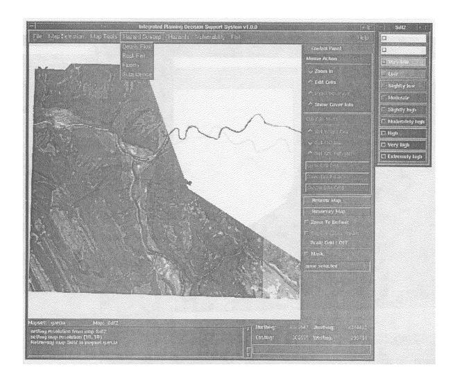
Figure 5. IPDS fourth step: selection of intrinsic 'Hazard Susceptibility' (Hs) to analyze with display of its algorithms and the possibility of editing these according to the user's judgement capabilities (results are normalized from 1 to 10).
