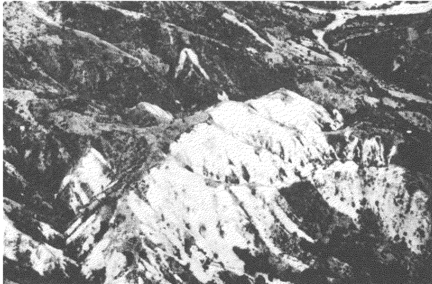
Figure 4.-- View of pumice slopes near Motagua River about 25 km north of Guatemala City which have suffered extensive failure and coalescence of debris slides. Debris slides are shallow, typically less than 1 m in thickness.
